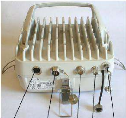
ETHERNET CONNECTOR ODU-ODU CONNECTOR PS CONNECTOR AGC CONNECTOR GROUND BOLT
